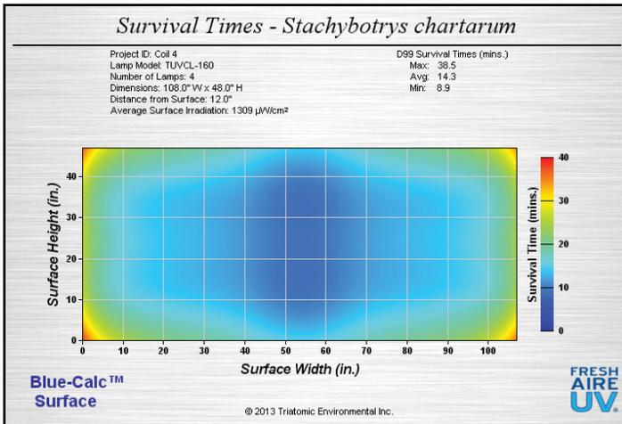
time consuming, and costly undertaking. Fortunately, UVGI systems can be mathematically modeled with fairly accurate results for the purpose of system sizing. Based on the system configuration and lamp parameters, the software models UV irradiance fields and determines microbe inactivation rates and times.
